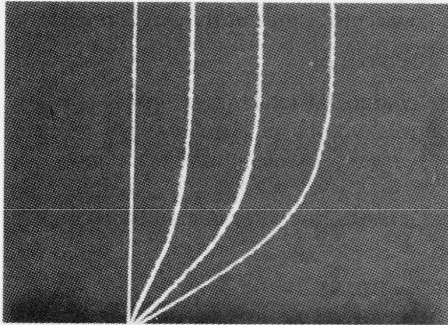
**Figure 5.8** Visualization of the longitudinal velocity profile in the laminar boundary layer over a flat plate: 0.01% salt water,  $U_\infty = 0.6$  cm/s, distance from the leading edge  $x = 20$  cm. (Nakayama et al. [12], with permission from Pergamon Press.)
