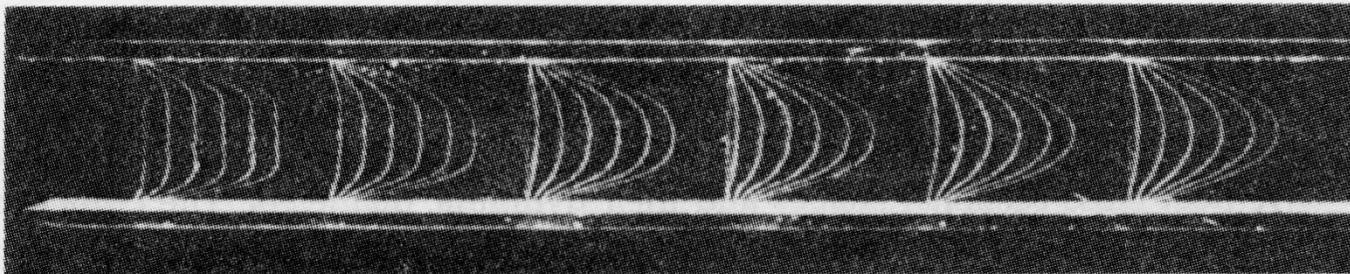
**Figure 6.4** Laminar flow in the entrance region of a parallel-plate channel: water,  $U = 3.2$  cm/s,  $D = 2$  cm. (Nakayama et al. [1], with permission from Pergamon Press.)
