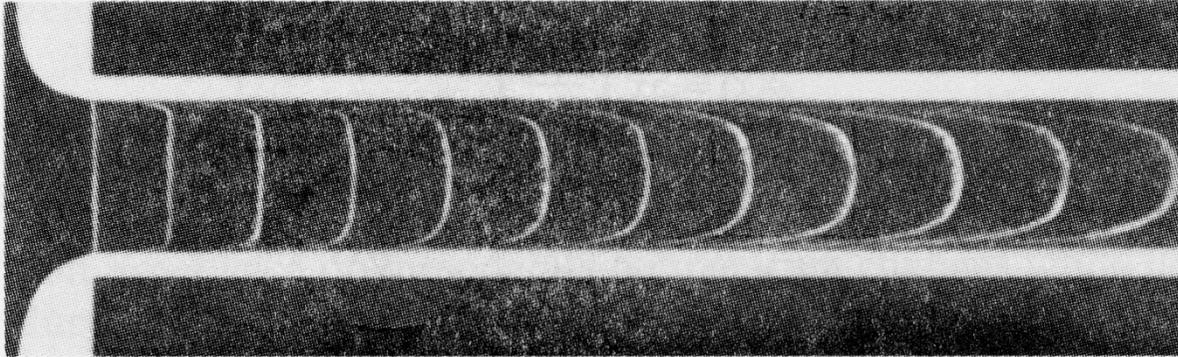
**Figure 6.2** Laminar flow in the entrance region of a tube with circular cross section: water,  $U = 6$  cm/s,  $D = 2.7$  cm. (Nakayama et al. [1], with permission from Pergamon Press.)
